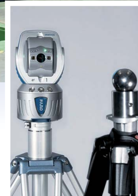
Sistema de medición laser tracker Measurement system by laser tracker
